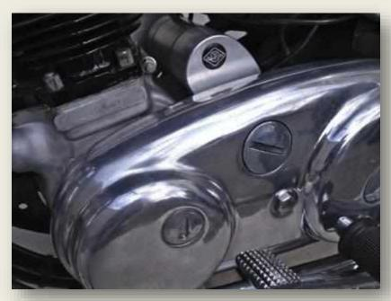
The Alton Electric Starter Kit for MK2 Commandos fits directly onto the engine via a specially designed inner chain case supplied with starter motor already mounted.
